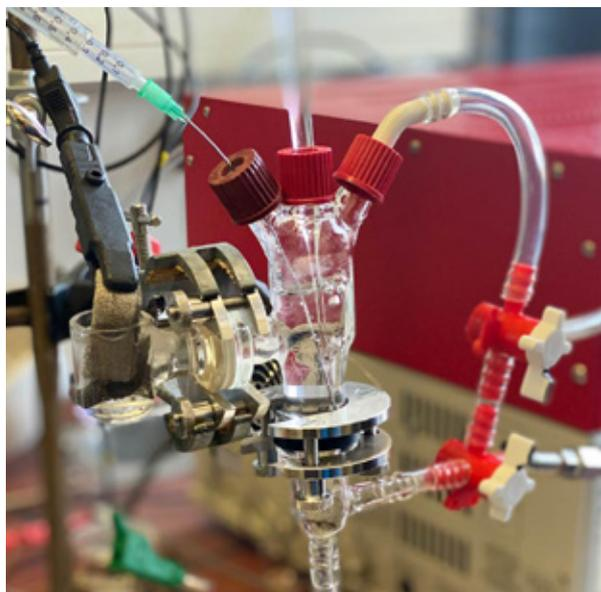
Laboratory test cell for catalyst screening.
